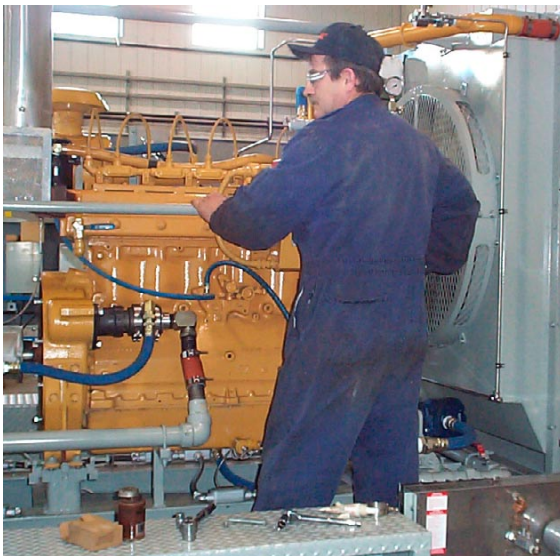
Pictured: ATS63-0312IT on Caterpillar G3306 natural gas package
